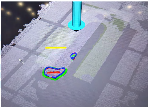
After blending, system executes a QA scan with a high resolution sensor and displays results as well as defect correction tool paths.
