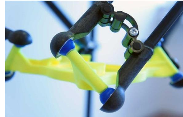
Thinking on where and how our customers need to place their robot in a work situation lead us to design an out of the box lightweight robot. Lightweight means rethinking the choice of materials without compromising performance. We replaced all possible parts with fiber-reinforced plastic on the RAGNAR Robot. Advanced thermoplastics and manufacturing delivers affordability without compromising quality and reliability. The result is a robot as light as 32kg!
