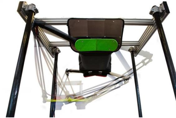
Traditional delta robots operate in a circular field limiting the workspace. The design of the RAGNAR Robot expands the operational workspace considerably, which means fewer robots can cover the same area more efficiently than traditional applications.
