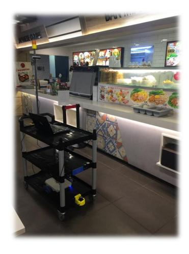
Developed to safely navigate in crowded environments. This trolley was meant to bring back the utensils from a tray return station to the washing area. To free the foodcourt staff from these duties.
