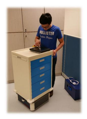
Developed a robotic system prototype to transfer safe and securely lab samples in a hospital environment. The system included scheduling and self charging.
