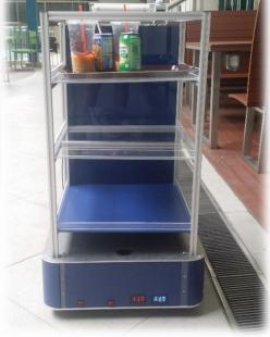
Developed a prototype for a proof of concept of tray returning robot in hawker centres in Singapore. Robot was developed and tested with SP open food courts.
