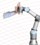
Teach by demonstration (Lead-through)
