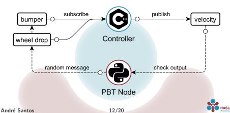
The setup for a PBT ROS node is always the same.
